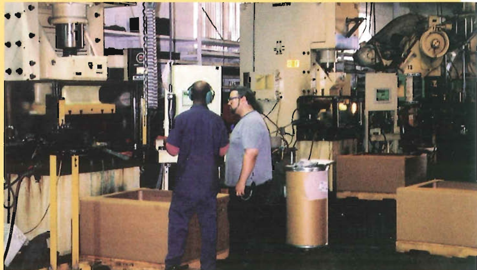
With controls and sensors in place, this operator can leave one press running unattended while he trains an employee on another.
